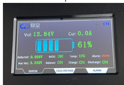
BMS monitor to view battery status. This is an option on some Lithium Batteries
