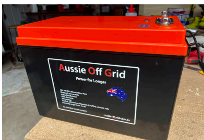
12V, 300Ah Lithium battery in a plastic case.
